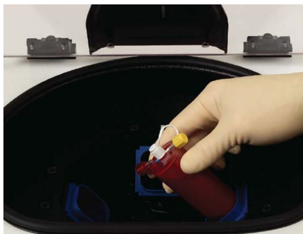
Fig. 3 GPS III system and centrifuge
